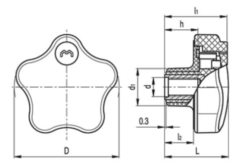
D = 41.5 d1 = 16.5 d 6H = M8 h = 13 L = 30 l1 = 29.5 l2 = 14.5 Weight (g) = 26
